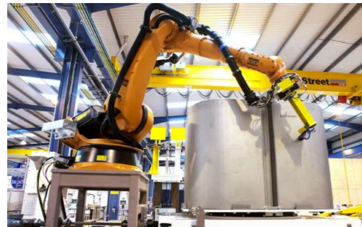
Robot Swabbing application. Robot completes swabbing of the cell. Swab is analysed for compliance with cleanliness standard.
