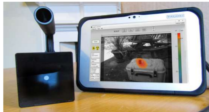
Mini Gamma Camera with SmartSpot™ software
