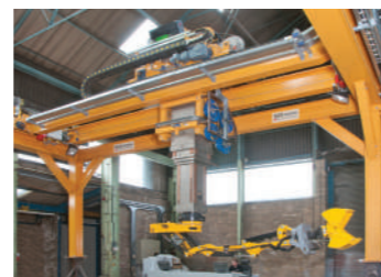
Extending mast & manipulator waste retrieval system
