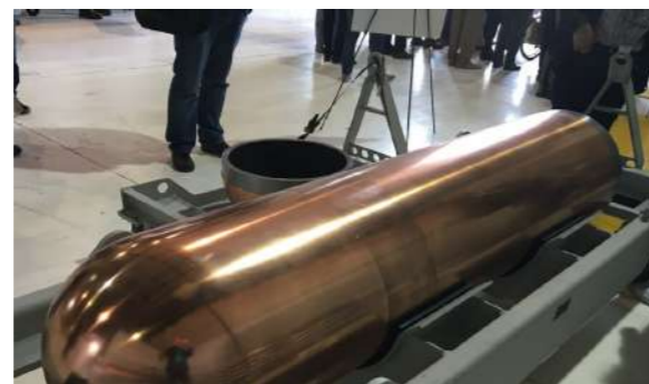
Copper coated high level waste containers
