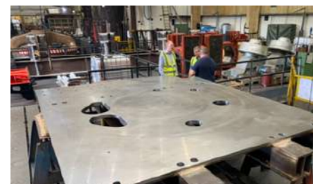
Support Structure for nuclear equipment
