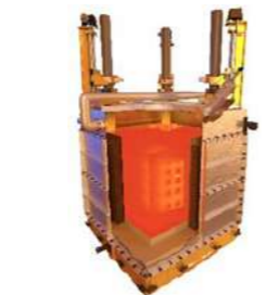
Cutaway of Geomelt Vitrification container
